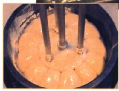
A 2kW Distromix B mixing a 10% guar gum slurry
