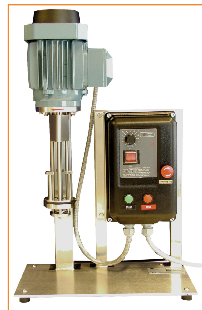
Example of custom DB50M system for pigment processing experiments
